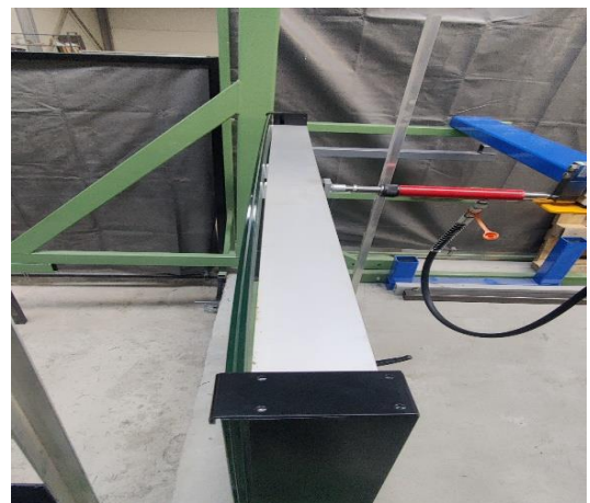
Figure 3: Balustrade during horizontal load test
