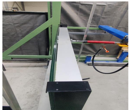
Figure 3: Balustrade during horizontal load test
